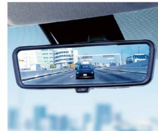
With camera monitor function enabled
